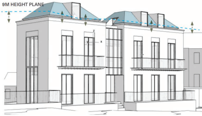
Figure 9: Perspective of the front elevation at 38 Lower Fort Street showing the 9m height plane parapet in dashed blue. (Source: Andrew Burns Architecture / Tasman Storey Architect)
